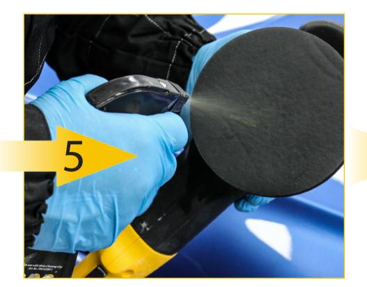
Action: Check edge definition of repair, making sure edges are beginning to blend. Dampen to reduce clouding. Use: Abralon P1000 and Mirka lubricant.
