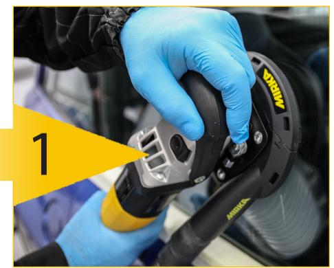
Action: Remove defects in the glass. **Use:** Abranet SIC NS discs grits P150 or finer through to P400. Always finish with P400.
