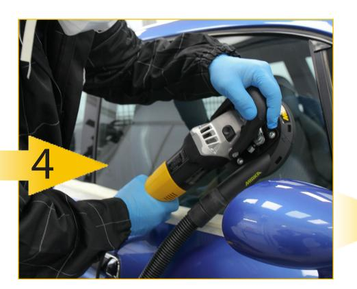
Action: During the Abralon stages, the machine must remain flat to help the edge blending process.
