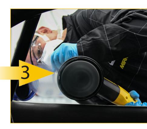
**Action:** Further reduce scracthes and repair edge. Expand the repair area with finer Abralon discs.
