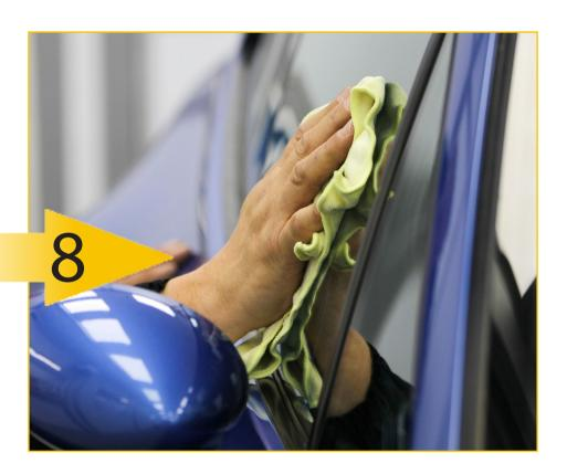
Action: Clean and inspect. Re-polish if needed for final result. **Use:** Mirka lubricant and microfibre cloth.
