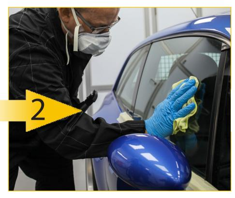
Action: Check and clean at each grit stage to be sure previous grits scratches have been removed.
