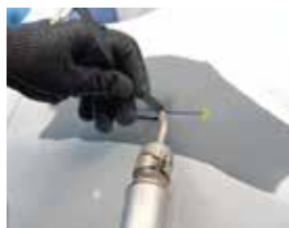
Splits and Cracked Bumpers
